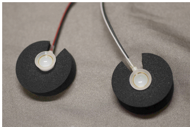
Fig.3 Electrode with holding sponge
